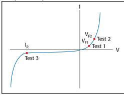
Pass/Fail Test If Passes Test If Fails Test Test Test 1 Check V<sub>F1</sub> at Go to Test 2 100mA against pass/fail limits 1. Bin part to bad bin Check V<sub>F2</sub> at 1A Go to Test 3 Test 2 against pass/fail 2. Transmit data to computer while limits handler is placing Test 3 Check leakage 1. Bin part to good bin new part current at -500V 2. Transmit readings to 3. Return to Test 1 and test against computer while handler pass/fail limits is placing new part 3. Return to Test 1
