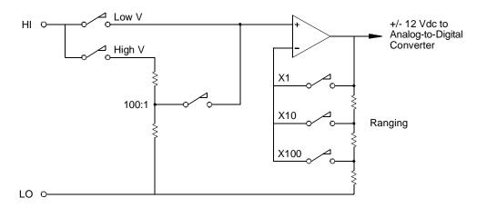
For input voltages less than 12 Vdc, the Low V switch is closed and applies the input signal directly to the input amplifier. For higher voltages, the High V switch is closed and the signal is attenuated 100:1 before being applied to the input amplifier. The input amplifier gain is set to one of three values (x1, x10, or x100) to yield a signal in the range of  $\pm 12$  Vdc for the analog-to-digital converter.
