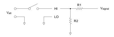
To select the attenuator components, use the following equation:
