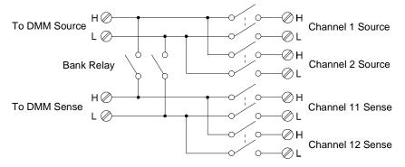
Note: If any channels are configured to be part of the scan list, you cannot close multiple channels; closing one channel will open the previously closed channel.
