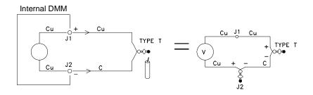
Notice, however, that the connections made between the thermocouple wire and the internal DMM make a second, unwanted thermocouple where the constantan (C) lead connects to the internal DMM's copper (Cu) input terminal. The voltage generated by this second thermocouple affects the voltage measurement of the T-type thermocouple.
