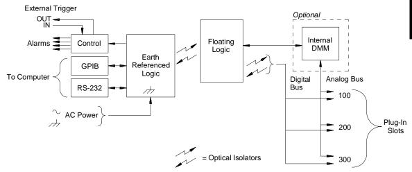
The earth-referenced and floating circuitry communicate with each other via an optically-isolated data link. The earth-referenced section communicates with the floating section to provide PC connectivity. The instrument is shipped with both an GPIB (IEEE-488) interface and an RS-232 interface. Only one interface can be enabled at a time.
