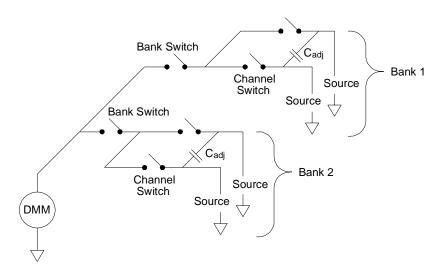
If you are not using all of the channels on the multiplexer, divide the input signals equally between Bank 1 and Bank 2. For example, if you are multiplexing eight channels using the 16-channel multiplexer, use four channels in the lower bank and four channels in the upper bank. For even better noise immunity, leave one unused, grounded channel between each input channel.
