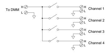
Note: Only one channel can be closed at a time; closing one channel will open the previously closed channel.
