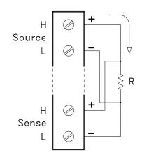
Channel *n* (source) is automatically paired with Channel *n*+10 (sense) on the 34901A or Channel *n*+8 (sense) on the 34902A.
