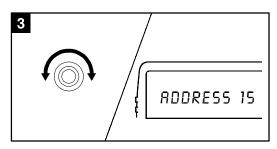
**3** Rotate the knob to view the choices on this level of the menu. When you reach the end of the list, rotate the knob in the opposite direction to view all of the other choices.
