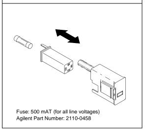
Rotate the line-voltage selector until the correct voltage appears in the window.
