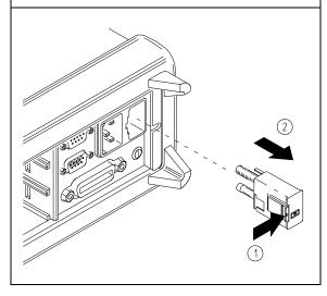
Remove the line-voltage selector from the assembly.
