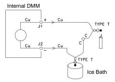
The T-type thermocouple is a unique case since one of the conductors (copper) is the same metal as the internal DMM's input terminals. If another type of thermocouple is used, two additional thermocouples are created. For example, take a look at the connections with a J-type thermocouple (iron and constantan):
