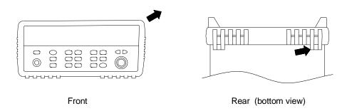
To remove the rubber bumper, stretch a corner and then slide it off.
