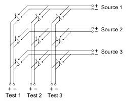
Any one of the signal sources can be connected to any one of the test inputs. Be aware that with a matrix, it is possible to connect more than one source at the same time. It is important to make sure that dangerous or unwanted conditions are not created by these connections.
