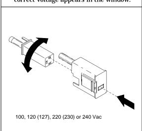
Replace the fuse-holder assembly in the rear panel.
