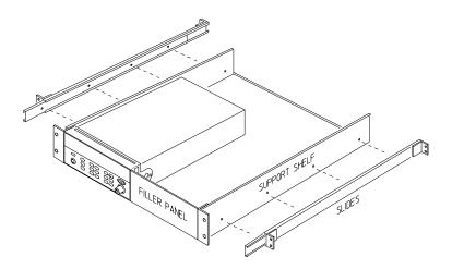
To install one or two instruments in a sliding support shelf, order shelf 5063-9255, and slide kit 1494-0015 (for a single instrument, also order filler panel 5002-3999).
