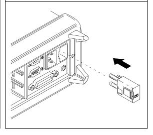
Verify that the correct line voltage is selected and the power-line fuse is good.
