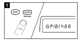
1 Press the menu key. You are automatically guided to the first level of the menu. Rotate the knob to view the other choices on the first level of the menu.
