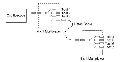
On the 34905A ( $50\Omega$ ) and 34906A ( $75\Omega$ ) RF multiplexers, you can close only one channel per bank at a time; closing one channel in a bank will open the previously closed channel. These modules respond *only* to the CLOSE command (OPEN does not apply). To open a channel, send the CLOSE command to another channel in the same bank.
