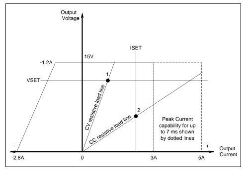
Figure 2-1. Dc Source Output 1 Characteristic
