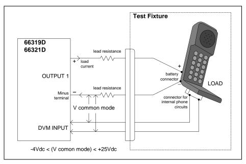
Figure 3-6. DVM Measurement Example
