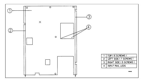
Figure C-4. Removing the Series 668xA/669xA Inner Cover
