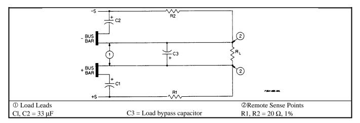
Figure 4-4b. Series 667xA Sense Lead Bypass Network
