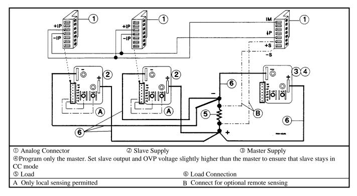
Figure 4-4e. Series 667xA Auto-Parallel Connection (Remote Sensing Optional)
