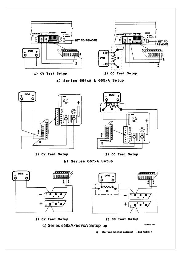
Figure A-1. Calibration Test Setup
