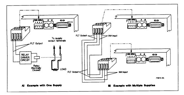
Figure D-3. Examples of FLT Outputs
