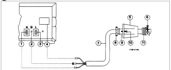
Figure 2-2. Connecting the Series 667xA Power Cord
