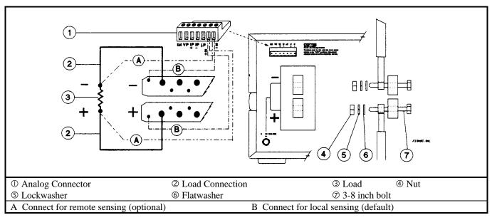
Figure 4-5c. Series 668xA and 669xA Single Load Connection (Remote Sensing Optional)
