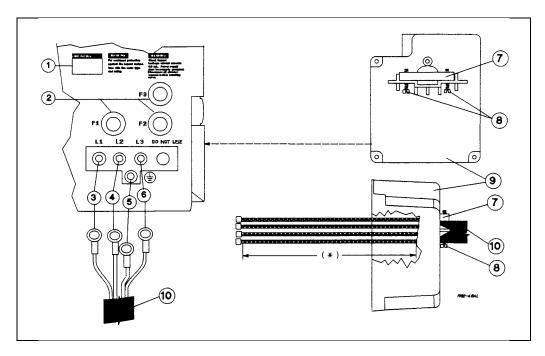
Figure 2-5. Connecting the Series 668xA Power Cord
