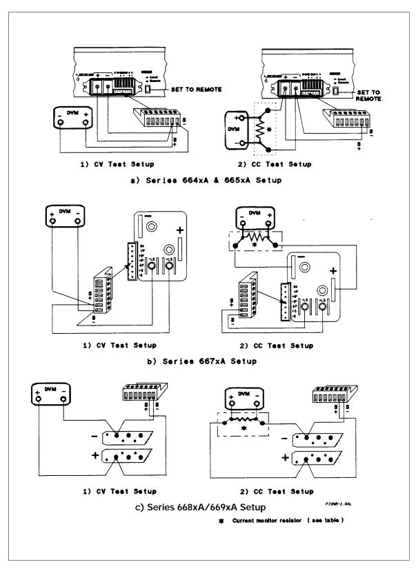
Figure B-1. Verification Test Setup
