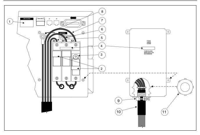
Figure 2-6. Connecting the Series 669xA Power Cord
