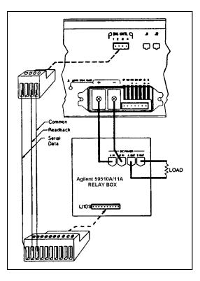
Figure D-6. Relay Link Connections
