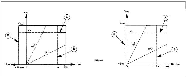
Figure 5-2. Typical Power Supply Operating Curve
