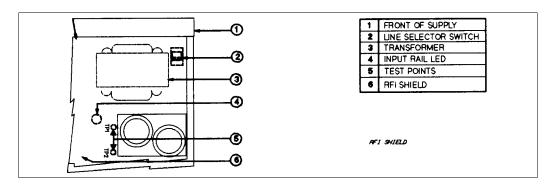
Figure C-3. Series 667xA Line Select Switch
