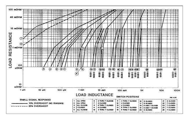
Figure E-1. CC Loop Compensation Curves for Models 6680A and 6681A
