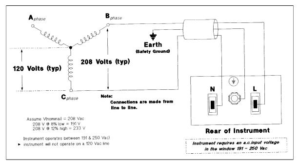
Figure 2-3. 667xA Connection to a 3-Phase Line
