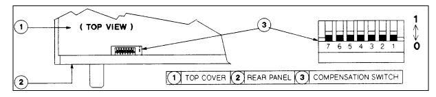
Figure E-2. CC Loop Compensation Switch
