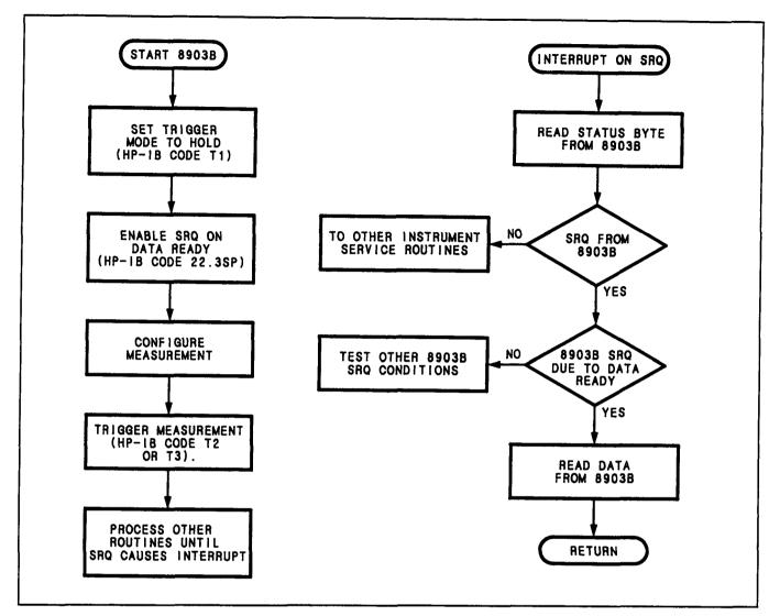
Figure 3-4. Example Flow Chart for Driving the Audio Analyzer Using the Require Service Message (SRQ)
