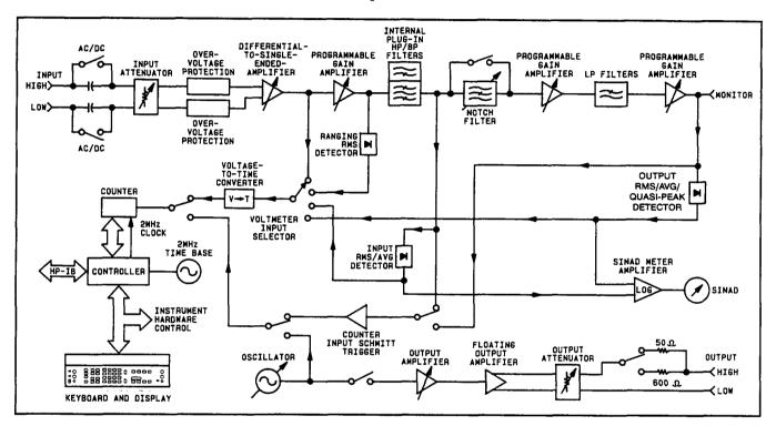
Figure 1-5. Simplified HP 8903B Audio Analyzer Block Diagram
