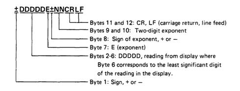
Data is always output in fundamental units (that is, Hz, %, dB, or V).
