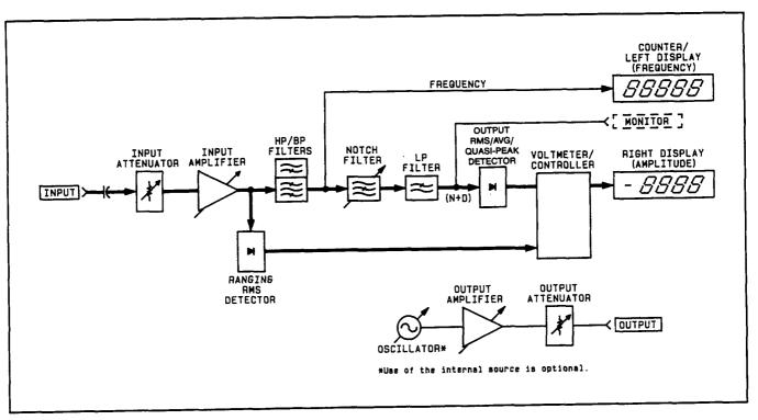
Distortion Level Measurement Block Diagram
