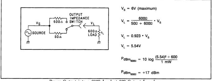
Power Output into a 600 $\Omega$  Load at 50 $\Omega$  Output Impedance
