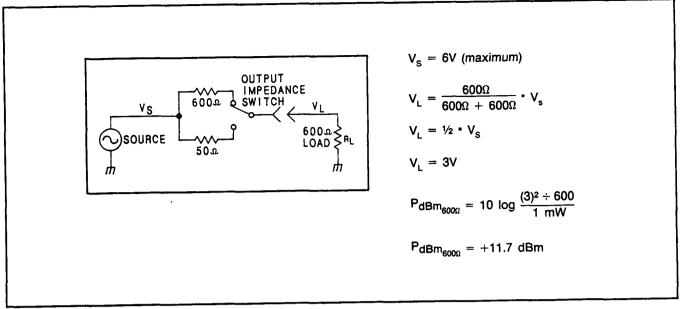
Maximum power Output into a 600 Load at 600 Output Impedance
