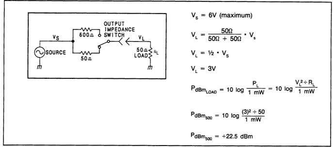
Maximum Power Output into a 500 Load at 500 Output Impedance
