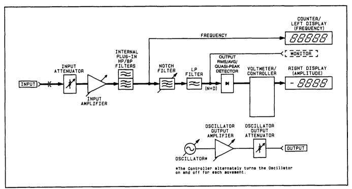
Signal-To-Noise Measurement Block Diagram
