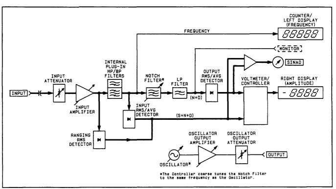
SINAD Measurement Block Diagram
