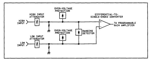
Analyzer Input Block Diagram
