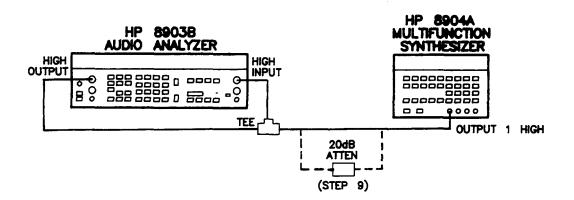
Figure 4-1. Distortion, SINAD, and Signal-to-Noise Accuracy Test Setup
