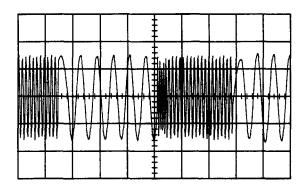
Figure 1-3. Two-Tone Burst Sequence (15 ms Duration)
