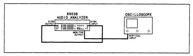
Figure 3-3. Basic Functional Checks Setup
