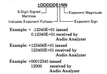
In general, do not issue numeric data with more significant digits than can be displayed on the Audio Analyzer's left five-digit display.
