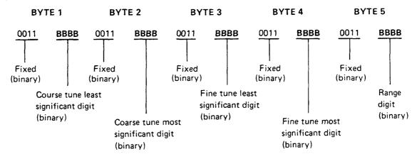
As shown above, the upper four bits of each byte sent to the Audio Analyzer are always 0011. This places the resulting codes in the ASCII range of "0" (decimal 48) to "?" (decimal 63). To build the five-byte sequence, convert the decimal data obtained via the Special Functions into binary. In the case of the coarse and fine tune data, split the eight bits into two groups of four (representing the most and least significant digits). Insert each four-bit packet into its respective byte.
