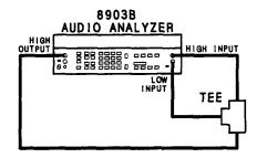
Figure 5-2. Common-Mode Rejection Adjustment Test Setup
