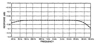
Figure 1-1. Typical Combined Source and AC Level Flatness
