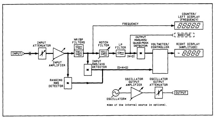
Distortion Measurement Block Diagram
