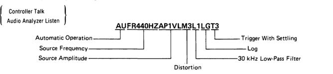
**Turning off Functions.** When operating in local mode, the High-Pass/Bandpass (optional plug-in filters), and Low-Pass Filters, and Ratio functions toggle on and off with successive keystrokes. In remote mode, these functions do not toggle on and off. Instead, each of the above groups has a specific code which turns off all the keys in the group. The HP-IB codes for turning off these functions are given in the following table.
