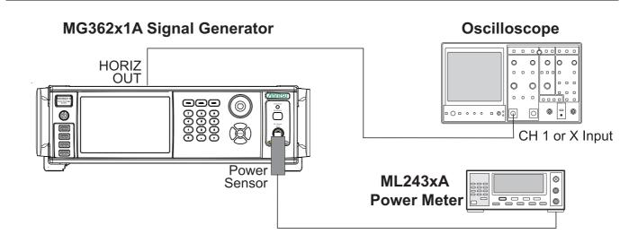
Figure 4-3. Equipment Setup for Accuracy and Flatness Tests
