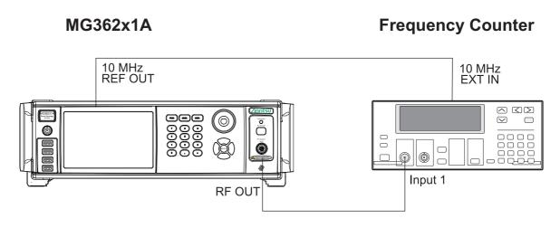
Figure 4-2. Setup for Frequency Synthesis Test
