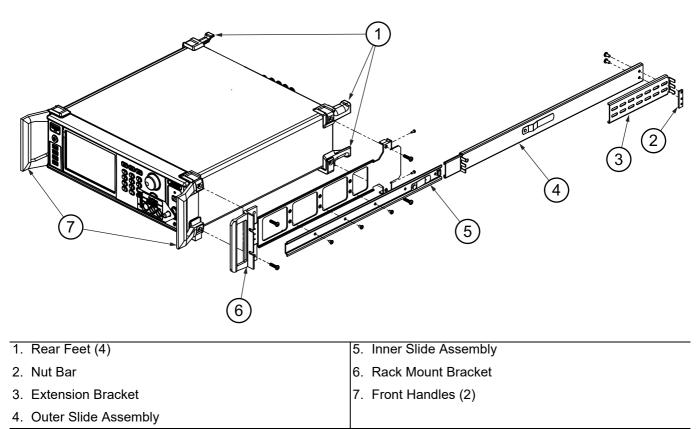
**Figure D-1.** Front Handle and Feet Removal
