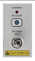
**Unleveled Indicator:** The unleveled indicator is displayed when the RF output goes unleveled and is normally caused by exceeding the specified leveled power rating.
