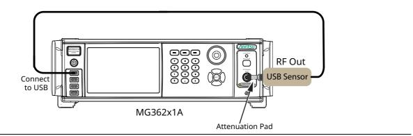
Figure 3-44. Internal Level Calibration Setup
