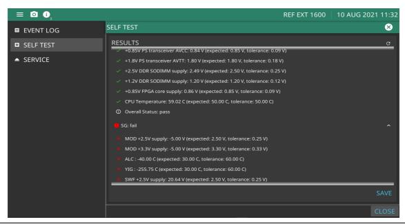
Figure 2-39. Self Test Status Log
