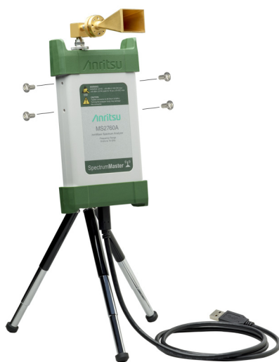
Figure 2-12. MS276xA Mounted to 1/4-20 Tripod (shows alternate M2.5 x 6.4 mm mounting screws)
