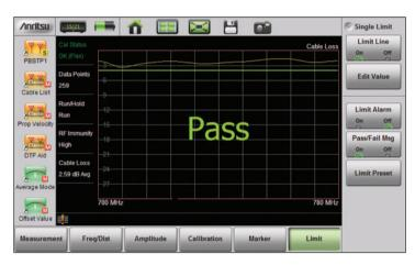
Cable Loss measurement screen (Advanced Mode)
