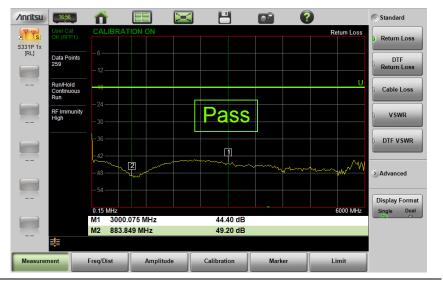
Figure 2-6. Return Loss Measurement
