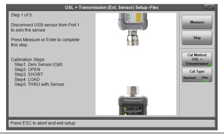
Figure 5-7. Transmission (Ext Sensor) Setup
