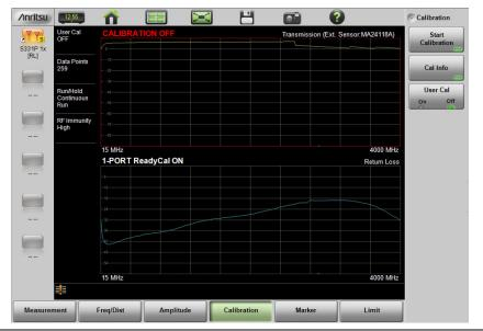
Figure 5-1. User Cal Off, ReadyCal On (All Measurements Except Transmission)
