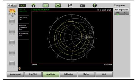
Figure 3-18. Set Reference Impedance for Smith Chart Calculations
