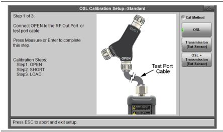
Figure 5-2. Calibration Method Selection
