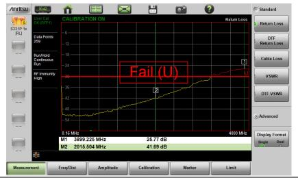
Figure 3-2. Failed Return Loss Measurement
