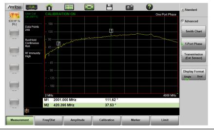
Figure 3-19. 1-Port Phase Measurement
