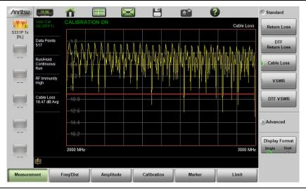
Figure 3-7. Cable Loss Measurement
