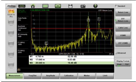
Figure 3-13. Failing DTF Return Loss Measurement (Antenna at 20.54 m)
