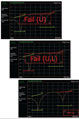
Figure 3-28. Pass/Fail Message Turned On
