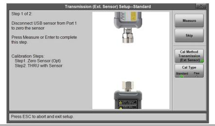
Figure 5-5. Transmission (Ext Sensor) Setup
