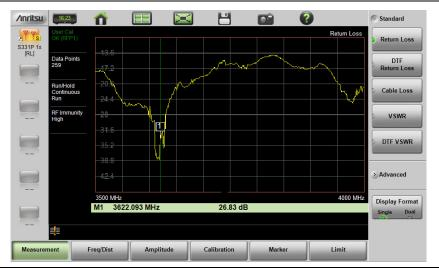
Figure 3-5. Antenna Return Loss Trace
