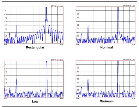
Figure 3-11. Effects of Windowing on a Sample Trace
