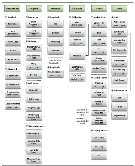
Figure 3-37. Cable & Antenna Analyzer Advanced Mode Menu Map
