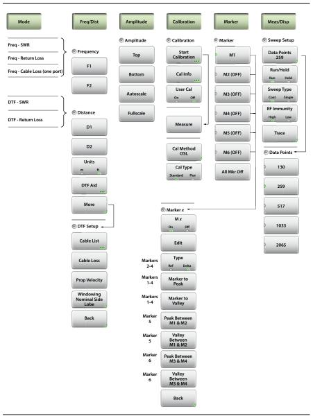
Figure 4-2. Cable & Antenna Analyzer Classic Mode Menu Map
