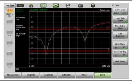
Figure 3-23. Limit Lines and Trace Showing Fail Colors
