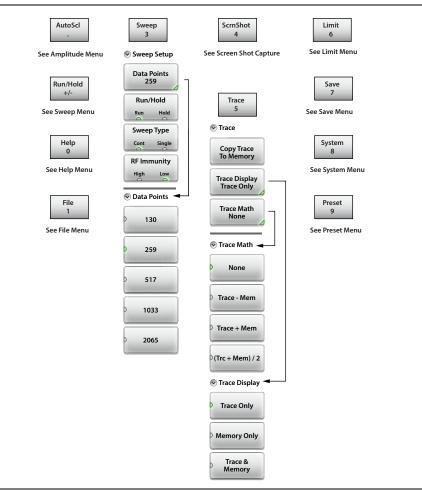
Figure 3-38. Virtual Keypad Function Keys
