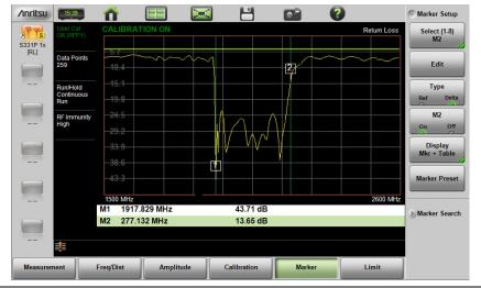
Figure 3-30. Delta Marker 2 and Marker Table
