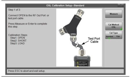
Figure 5-3. OSL Calibration Setup
