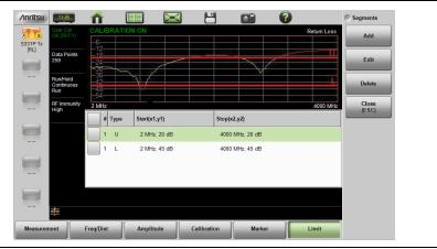
Figure 3-24. Table of Limit Lines (or Segments)
