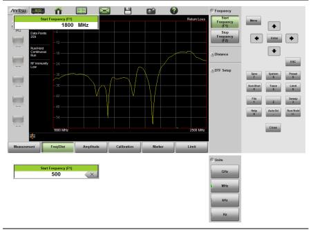
Figure 3-21. Entering Frequency Setting
