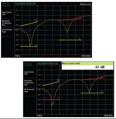
Figure 3-27. Moving Limit Line Segments
