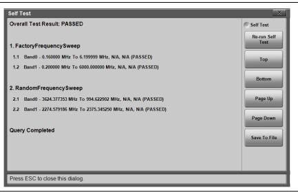
Figure 7-4. Self Test Window
