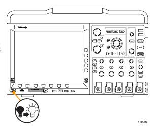
**5.** Power off the oscilloscope and remove the USB flash drive.
