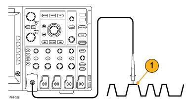
**2.** Select the input channel by pushing the front-panel buttons.
