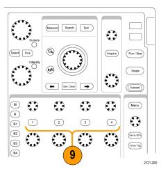
10. B1 or B2. Push to define and display a bus if you have the appropriate module application keys. The DPO4AUTO module supports CAN and LIN buses. The DPO4AUTOMAX supports CAN, LIN and FlexRay buses. The DPO4EMBD module supports I<sup>2</sup>C and SPI. The DPO4COMP module supports RS-232, RS-422, RS-485, and UART buses.
