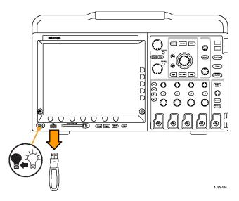
6. Power on the oscilloscope.
