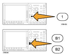
2. Push a lower-bezel button to create a label, such as for channel 1 or B1.
