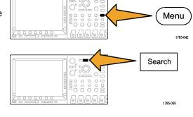
10. Push Search Type. Use the multipurpose knob a to select Bus and then push Data. Use the multipurpose knobs a and b to define the data value.
