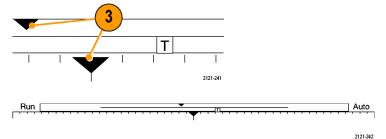
4. The waveform record view shows the trigger location relative to the waveform record. The line color corresponds to the selected waveform color.
