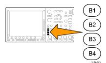
Push the Bus Display lower-bezel button, push the Bus and Waveforms side-bezel button, and push the ASCII side-bezel. Turn the Horizontal Scale knob to adjust the timebase.
