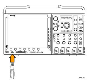
Power on the oscilloscope. The instrument automatically recognizes the replacement firmware and installs it.
