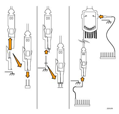
2. Connect the ground lead or leads to the circuit ground.
