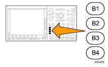
Push Bus. Turn multipurpose knob a to scroll through the bus type side menu until you select the desired bus: Parallel (MSO4000 series only), I<sup>2</sup>C, SPI, CAN, RS-232, LIN, or FlexRay. The actual menu items shown will depend on your model oscilloscope and the application modules installed.
