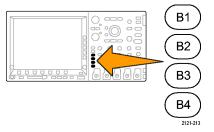
**2.** Turn multipurpose knob **a** to adjust the vertical position of the selected bus.
