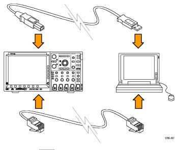
To communicate between the oscilloscope and a GPIB system, connect the oscilloscope to the TEK-USB-488 GPIB-to-USB Adapter with a USB cable. Then connect the adapter to your GPIB system with a GPIB cable. Cycle the power on the oscilloscope.
