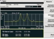
TOI – Easily quantify distortion performance. With the automated third order intercept measurement, you can conveniently quantify the intermodulation immunity of your device.
