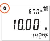
icon will flash when the instrument is connected to a mobile device.
