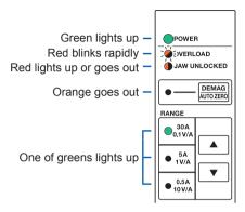
The input current exceeding the specified level of each current range is detected.
