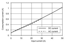
Fig. 7 Consumption current (with the 30 A range specified)
