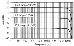
Fig. 1 Frequency characteristics (Model CT6710)
