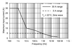
Fig. 3 Derating curve according to frequency (Model CT6710)
