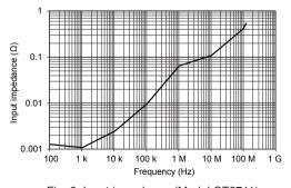
Fig. 6 Input impedance (Model CT6711)
