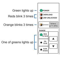
Demagnetizing and automatic zero-adjustment cannot be performed; otherwise, demagnetization or automatic zeroadjustment has not been completed normally.
