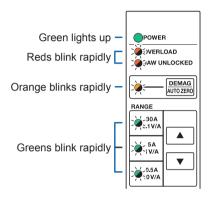
The abnormal internal temperature was detected in the junction box, and thus the device has entered protection mode.
