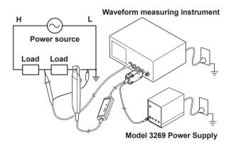
Model 3269 can provide the power to up to two probes of Model CT6710/CT6711.
