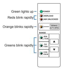
In protection mode, the device cannot correctly measure any current. Moreover, you cannot switch the current ranges. When the device has entered protection mode, follow the procedure presented in the following pages to restore it to normal operation.
