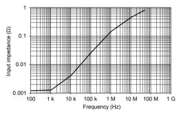
Fig. 5 Input impedance (Model CT6710)
