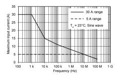
Fig. 4 Derating curve according to frequency (Model CT6711)
