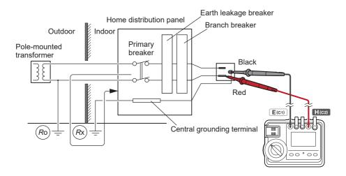
Always execute a zero adjustment before measurements. (p.82)
