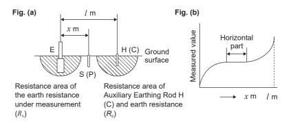
Electrodes E and H (C) can be separated up to 50 m by using the optional L9843-51, L9843-52, or L9843-53. Electrode S (P) can also separated from Electrode E within the distance where the horizontal part is found shown in Fig. (b). Measurements can be made, in principle, even if they are separated more than 50 m; however, the measurement results cannot be guaranteed.
