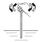
Hold the loop part of an auxiliary earthing rod with your hand and pull it out while turning it.
