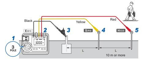
Disconnecting the earth electrode from the installation allows the instrument to measure earth-resistance values correctly. Disconnect the earth electrode from the installation before staring a measurement. If the earth electrode cannot be separated from the equipment, make measurements using the three-pole MEC measurement.
