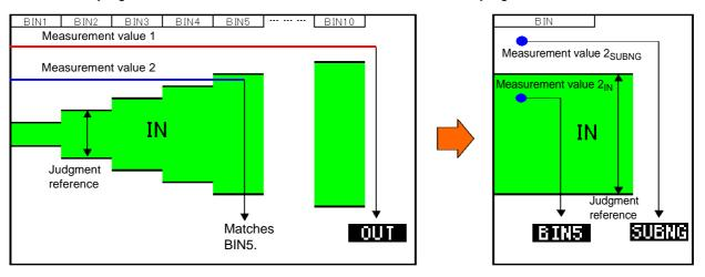
In BIN judgment, a judgment is made based on the main measurement value first, and then the result of a judgment using the sub measurement value is output. In the above example, is displayed since main measurement value 1 did not fulfill any of the set judgment standards. Main measurement value 2 was the first to fulfill the standard, and **SUBJE** is displayed since the judgment standard set for BIN5 was fulfilled.
