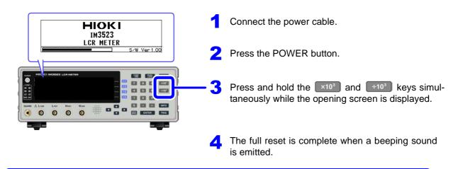
If the instrument still does not operate normally after the full reset, it needs to be repaired. Contact your dealer, or a Hioki representative if you are not sure where the instrument was purchased.
