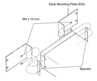
Installing the spacers on both sides of the instrument, affix the Rack Mounting Plate with the M4 x 10 mm screws.
