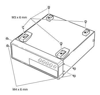
Remove the feed from the bottom of the instrument, and the screws from the sides (four near the front).
