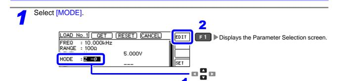
6.3 Adjusting Values Based on Reference Values(Load Compensation)
