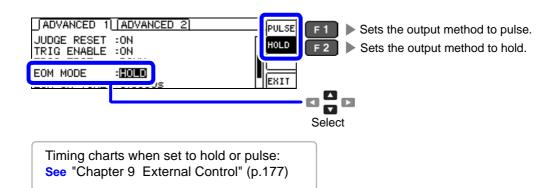
Select [EOM-ON-TIME] and set the EOM output time to use with pulse EOM mode. Settable range: 0.0001 s to 0.9999 s
