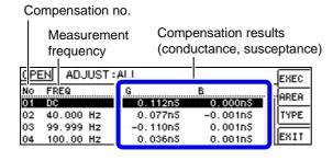
When compensation completes normally, the conductance and susceptance will be displayed. Compensation is supported for impedance values of 1 k $\Omega$  or greater.
