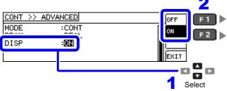
Turns off the backlight when there has been no key operation for about 10 seconds.
