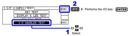
Perform the output signal test and input signal test.
