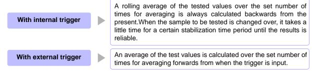
When the number of averaging times is 4, the number of measurements, measurement output points, and measurement value calculation method during output are as follows.
