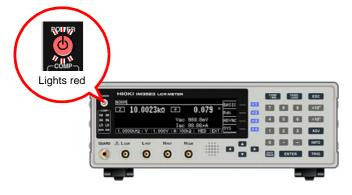
Disconnect the power cord from the outlet to extinguish the POWER button light.
