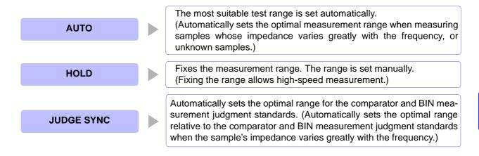
The ranges are all defined in terms of impedance. Therefore, for a parameter other than impedance, the value is obtained by calculating from the measured values of |Z| and  $\theta$ . See "Appendix1 Measurement Parameters and Calculation formula"(p. A1)
