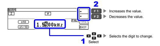
NOTE The digits in the measurement frequency can also be changed using the \textbf{\textsuperposition} keys.
