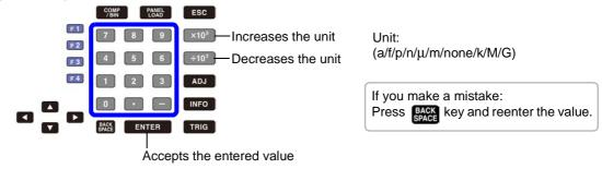
When entering a value for compensation coefficient A, the x103 keys are disabled.
