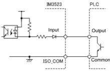
PLC Input (Sink Input) Connections
