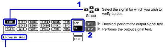
The names of signal lines that are being input (low) are shown in the input signal test window.
