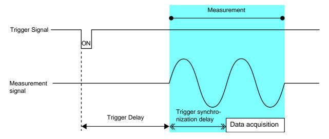
**NOTE** When the range synchronization function has been set, the range settings at which the trigger delay and trigger synchronous output function are enabled vary with the parameter settings.
