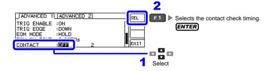
Select the timing at which to perform contact check operation.
