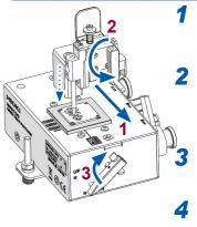
Using the pusher sideways knob, move the pusher unit to the location of the sample.
