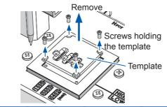
Attaching the short correction jig and performing correction
