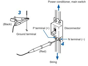
There is a risk of insulation deterioration when voltage is generated between the N terminal and ground. When there is voltage in the object under measurement, the backlight blinks in red by the voltage detection function.
