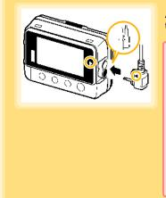
Align the triangle on the plug with the one in front of the sensor jacks, and insert the plug securely.
