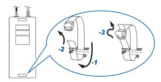
Attach the strap buckle to a compatible instrument and connect it to the clip that you attached to the device with the strap.
