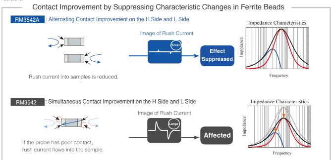
[Low-impact Contact Improvement Conditions] LOW POWER: ON or Applied Voltage Limit Function: ON, and Contact Improver Function set to Pulse.
