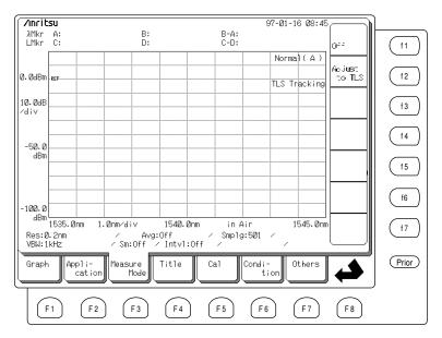
If the message "TLS Interface Error" is displayed at this time, check the cable connections again and the MG9637/MG9638 settings.
