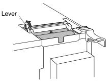
(4) Check that the paper alignment is straight. Return the lever to its original position as shown by the arrow in the following diagram. Turn the paper feed Knob to feed the paper and replace the printer cover.
