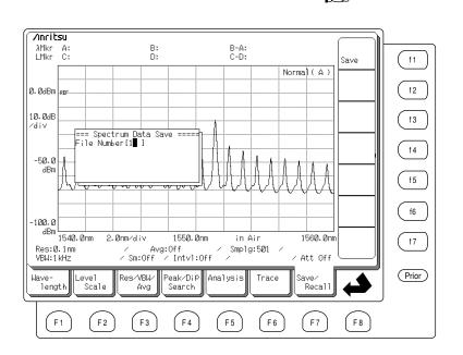
This example explains how to save the data to file number 1. When 1 is input as the file number, a file called "data001.dat" is created on the FD. The name of the file created at this time may be different such as "data001,bmp" or "data001.txt" depending on the File Option settings of Save/Recall card.
