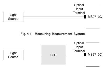
Fig. 4-2 Measuring Device Under Test
