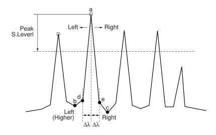
The peak level Lp [dBm] detects the value of peak point a. The peak wavelength  $\lambda p$  is the wavelength of peak a when Peak Type of Peak Prmtr is set to MAX and the half-width center wavelength of the peak when Peak Type is set to Threshold.
