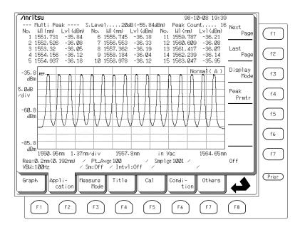
There are four display modes for WDM signal analysis: Multi Peak, SNR, Relative, and Table, and the displayed items are different in each mode.
