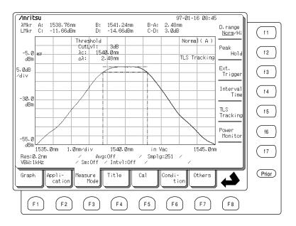
Note that during tracking measurement, the Auto measurement and the W1 Offset function key  $(f_1)$  of the Cal card selected by pressing  $(f_5)$  key is not passible to be used.
