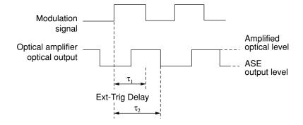
To measure the amplified optical level the Ext. Trig Delay should be set to  $\tau_1$ . The ASE output level is measured when the Ext. Trig Delay is set to  $\tau_2$ .
