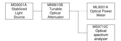
(a) Connect the tester and measuring instruments as shown below.
