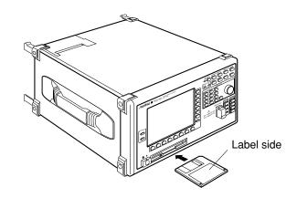
The FDD can be used at ambient temperatures of 5 to 50 °C.
