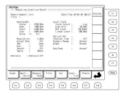
Select the desired Memory Number at the top left of the screen, then press the Execute function key  $(f_1)$  to recall the measurement conditions. When Memory Number 0 is selected, the factory default memory conditions are recalled.
