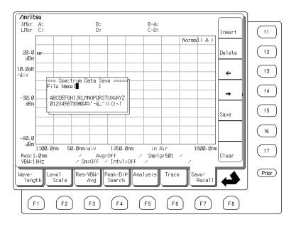
The following function keys are displayed in the Functions display field at right-hand side of the screen.
