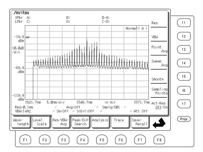
Press the Peak $\rightarrow$ Ref Level (RefLv) of shortcut keys to set the peak level to the reference level.
