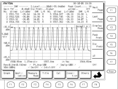
In the SNR mode, the wavelength, level, and SNR of up to 8 peaks can be displayed simultaneously.
