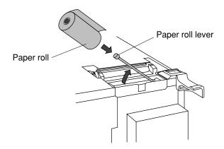
(3) Push the lever in the direction shown in the diagram below and feed the end of the paper between the print head and the platen.
