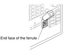
(4) Carefully refit the optical input connector taking care not to scratch or otherwise damage the end face of the ferrule.
