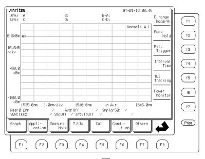
Press the Adjust to TLS function key (f2) then select Execute by pressing the function key (f1), which sets the measurement conditions automatically and start calibration. Calibration of the tracking wavelength will take about a few minutes.
