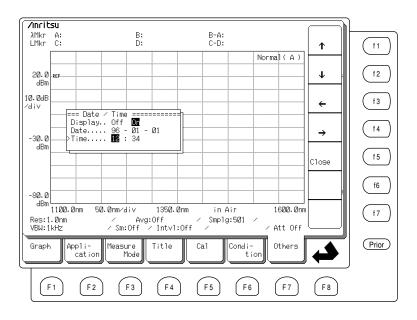
The following function keys are displayed in the Functions display field at right-hand side of the screen. Use the function keys to select the item indicated by the reverse displayed cursor.
