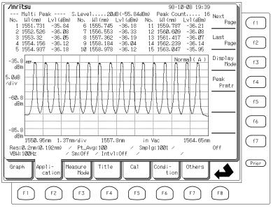
In the Multi Peak Mode, the wavelength and level of up to 15 peaks can be displayed simultaneously. Next page displays the following page.
