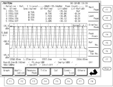
In the Relative mode, the wavelength, level, and wavelength spacing, or the wavelength and level relative to a reference peak, can be displayed for up to 5 peaks simultaneously.
