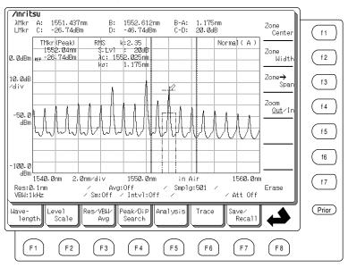
This Zone Marker function is useful for analyzing a specific spectrum individually while monitoring several spectra simultaneously as in WDM applications, etc.
