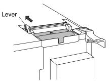
(5) Press the lever in the same direction as in step (2). This completes the paper change.
