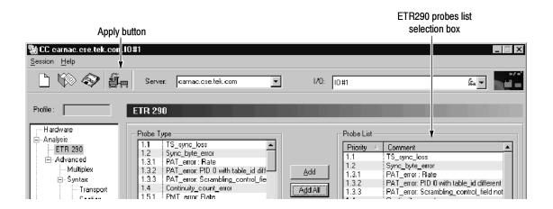
Figure 2-18: Setting ETR290 probes
