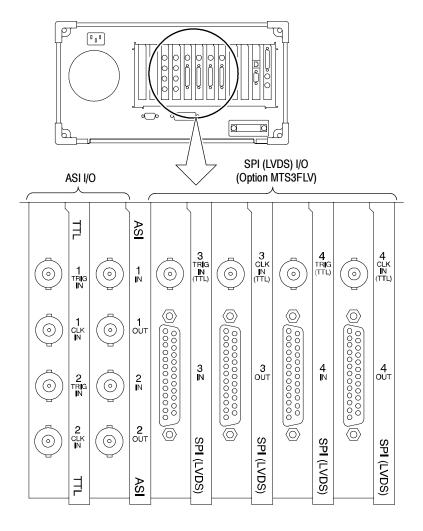
Figure 1-3: MTS300 inputs and outputs
