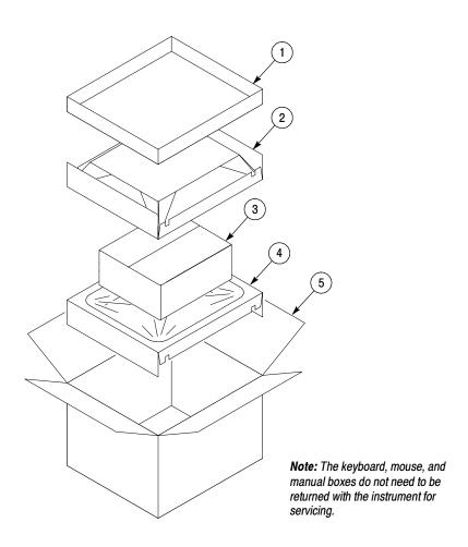
Figure B-2: Repackaging the instrument (old packaging)
