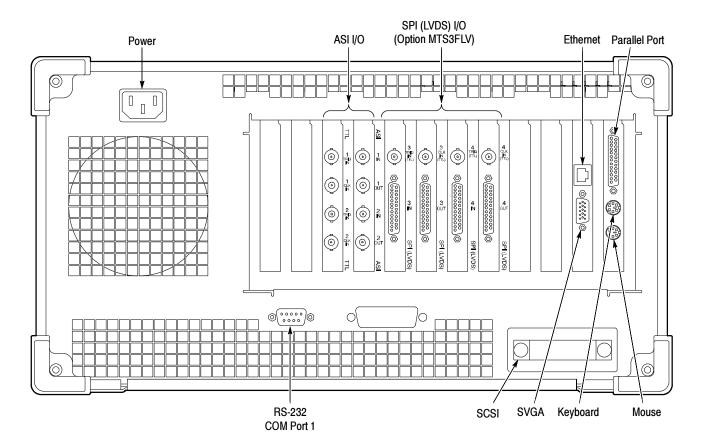
Figure 1-2 shows the locations of the connectors on the MTS300 rear panel.
