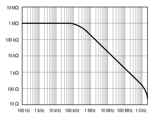
Figure 3–3: Typical Input Impedance vs. Frequency
