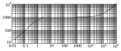
Figure 2-8. OC-N Mask to use with Generating Phase Transient
