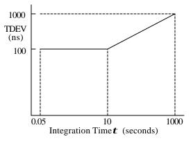
Figure 2-12. Wander Tolerance GR-1244-CORE Fig. 4-2
