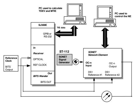
Figure 2-7. SONET OC-N Phase Transient Specification conformance testing.
