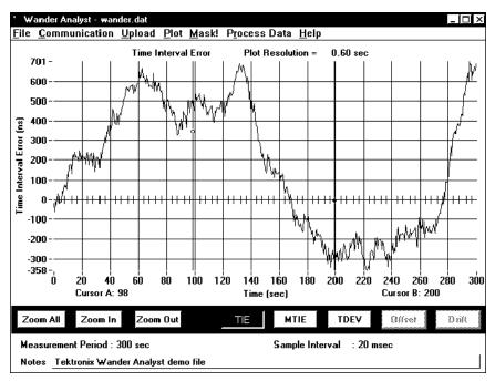
Figure 2-18. TIE phase characteristic of wander noise test signal (G.813 input tolerance test signal)
