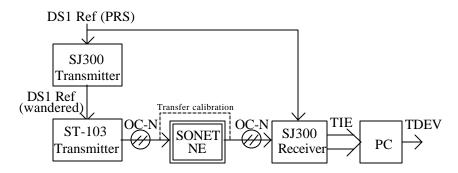
Figure 2-11. Setup for Testing Conformance to Wander Transfer Specification R5-126.
