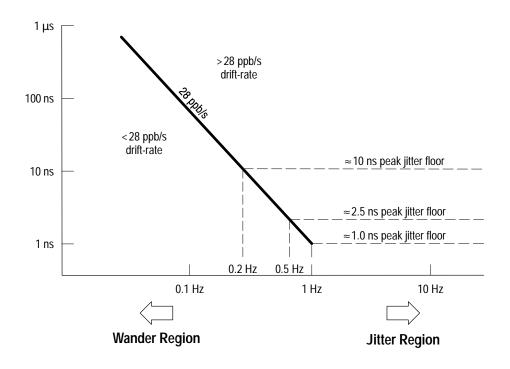
Figure 5: Plot of time error versus frequency accommodation
